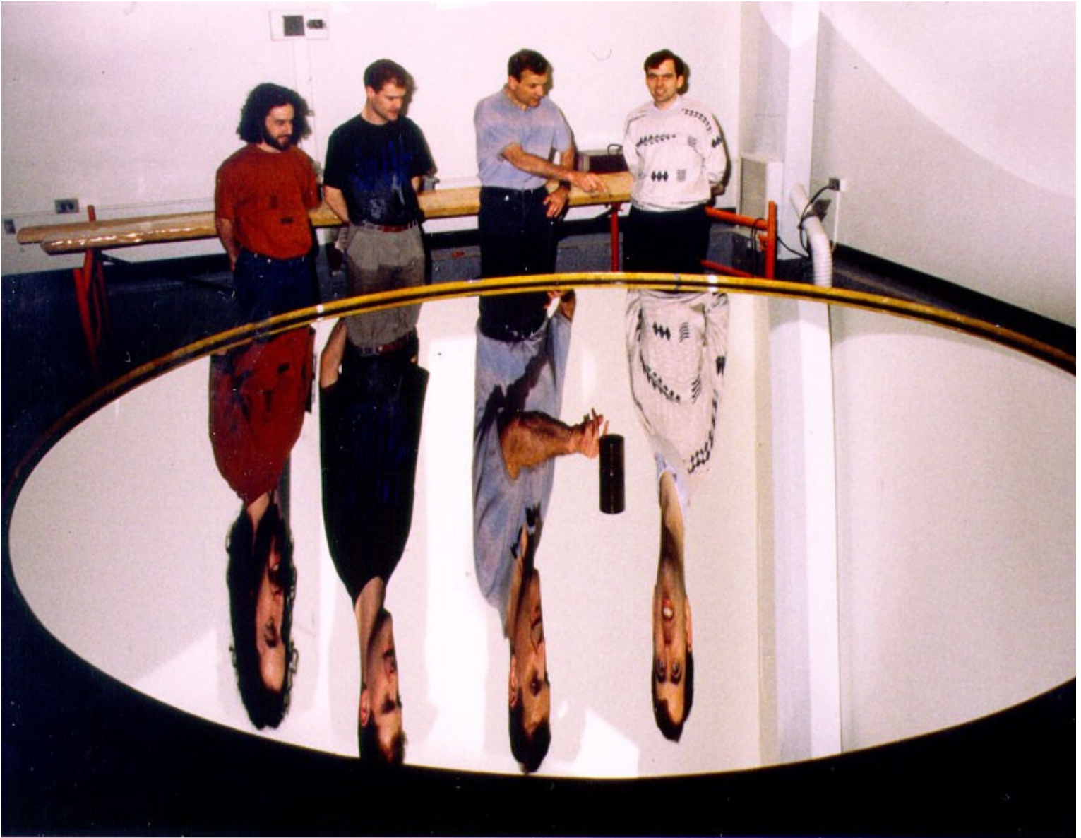
A 3.7 meter diameter liquid mirror at Université Laval in Quebec, Canada. The liquid is mercury. There are no detectable mercury because a thin transparent layer of oxide covers the surface. (Image Credit: Guy Plante, Université Laval)
