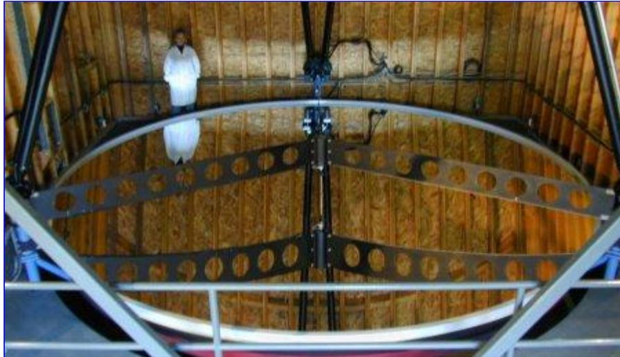
Much less dense than mercury, ionic liquids are only slightly denser than water. Although not highly reflective themselves, a spinning mirror of an ionic liquid can be coated with an ultrathin layer of silver just as if it were a solid mirror. Weirdest of all, the silver layer is so thin—only 50 to 100 nanometers—that it actually solidifies. In the vacuum of space, a liquid mirror coated with a thin solid layer of silver would neither evaporate nor tarnish.
