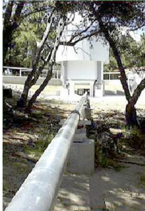
One of the six 1-meter telescopes making up the CHARA Array. Light from each scope is sent through a vacuum pipe (foreground) to a central facility. Here individual light waves, sampled by telescopes up to 330 meters apart, are delicately reassembled — enabling the array to measure angular sizes as small as 0.2 milliarcsecond for bright objects. Courtesy CHARA / Georgia State University.
