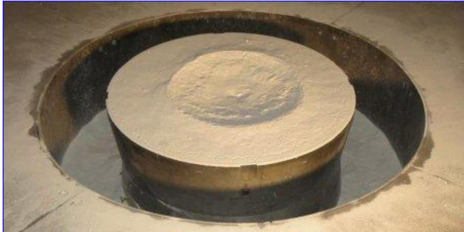
**Above:** A 30cm-diameter crater plus spattered dust are all that's left after a test shot in the Ames Vertical Gun. Photo credit: NASA. [[Larger image](#)]
